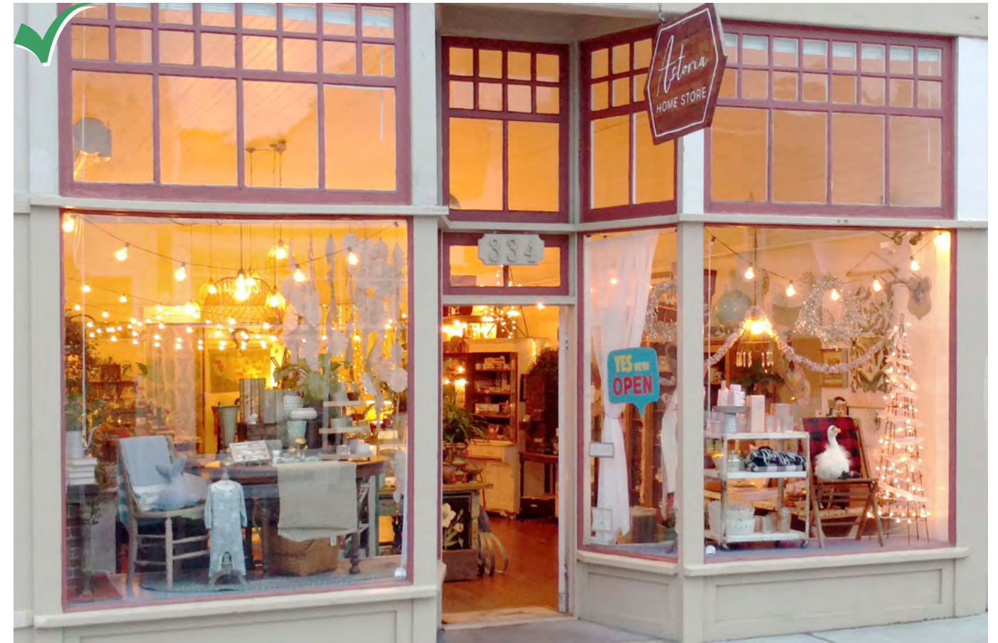
Create and maintain large, glass, street-level storefronts with 50-80% or more of their area open. Limit window obstructions to de-clutter windows and provide interior views. Recessed entryways offer protection from the elements.
